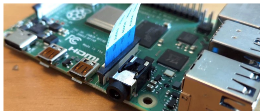
Abbildung 4: Raspi Cam Slot am Raspberry Pi
